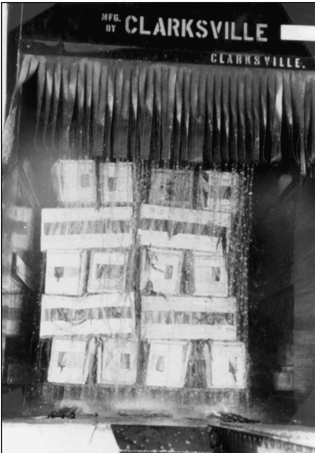
Figure 2. Conveyor hydrocooler precooling palletized crates of sweet corn.
