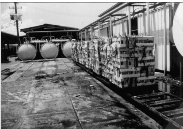
Figure 1. Vacuum cooler chambers and palletized crates of sweet corn.
