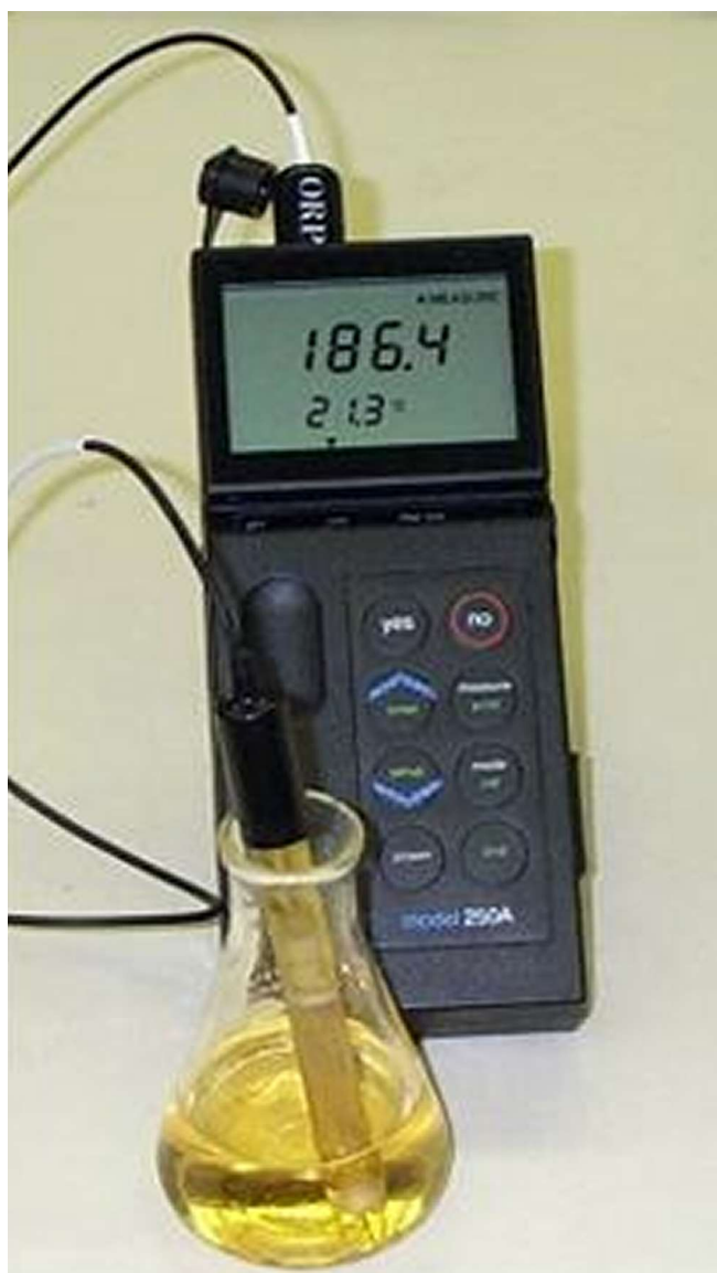
Figure 9. A handheld ORP/pH meter with ORP probe reading a standard.
